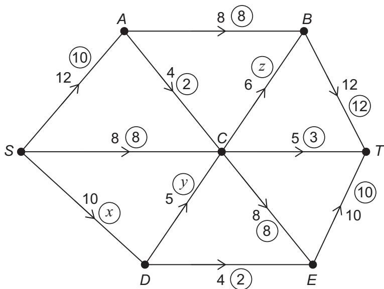
The uncircled numbers on each arc represent the capacity of each pipe in  $\text{m}^3 \text{ s}^{-1}$
