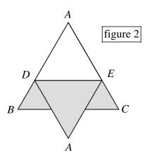
A uniform lamina ABC is the shape of an isosceles triangle where AB = AC, BC = 6a. The vertical height of ABC is 9h, as shown in figure 1. The lamina is to be folded along DE, where DE is parallel to BC and at a perpendicular distance of 6h from A, as shown in figure 2.
