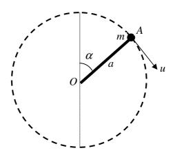
One end of a **light** rigid rod, of length a, is freely jointed to a fixed point O and the other end is attached to a particle of mass m.
